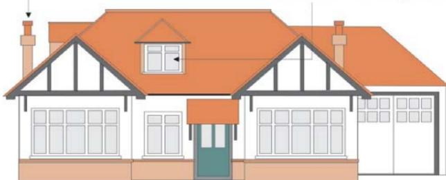
dormers on the front and side elevations should be small and unobtrusive and substantial roof slopes should be maintained either side of the dormer
